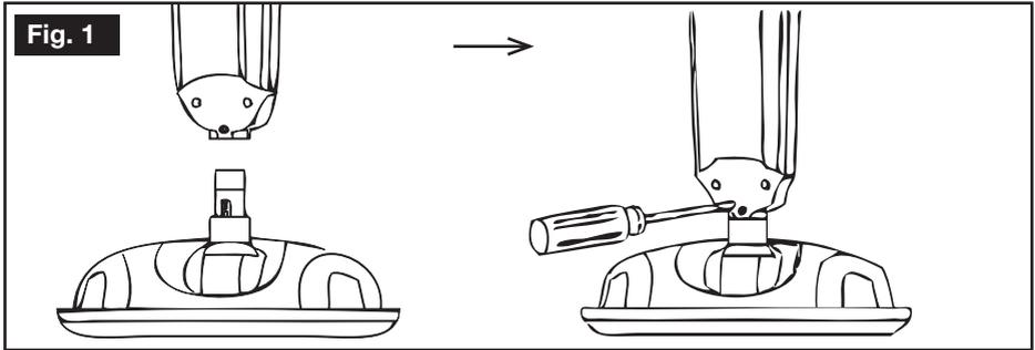
2. Following the illustrations below, insert the handle into the body of the steam mop (Fig. 2). Make sure to insert it fully so the screw hole in the handle is aligned with the screw hole in the body of the appliance.
