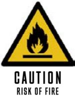
This symbol alerts you to take care as this beverage chiller contains a flammable refrigerant (isobutane) and insulation blowing gas (cyclopentane). Do not expose it to high heat, sparks and open flames.
